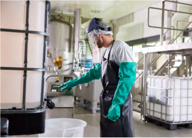
Safe weighing of hazardous substances in production, Kehl, Germany. Adherence to necessary personal protective equipment ensures employee and environmental safety.
