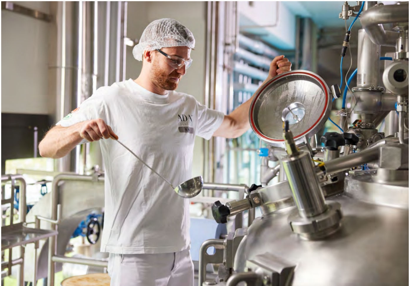
Maintaining high-quality standards: Regular drawing of samples of the bulk from the mixing vessel allows employees to check and ensure consistent quality throughout the production process.
